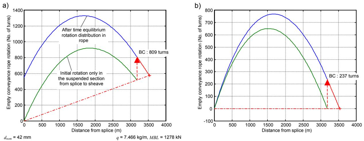
**Figure 8** - Calculated rope rotation distributions after installation resulting in a conveyance end lay length of nominal -20 % and a sheave end lay length of nominal +45 %. a) Rope closed at nominal +3.7 % and 550 unlaying turns released after installation. b) rope closed at nominal +10 %, no rotation released after installation. The rotation boundary conditions (BC) at the sheave after achieving twist equilibrium from the sheave to hawse hole are shown.
