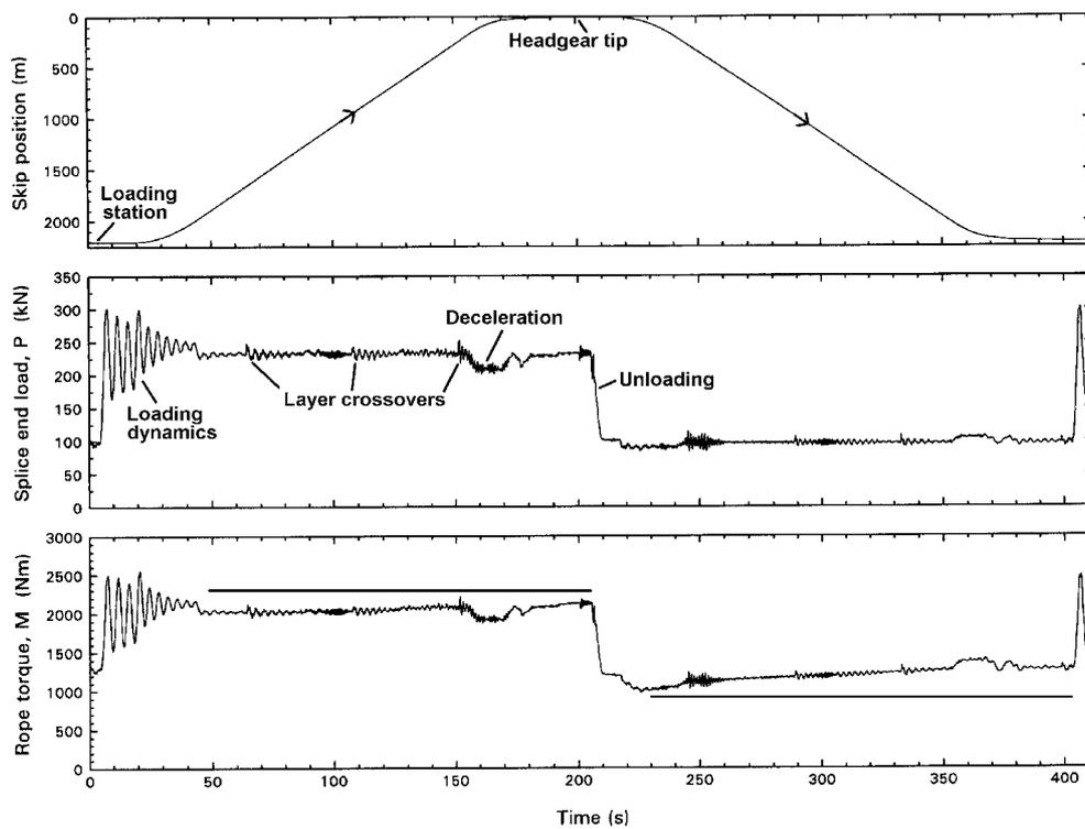
**Figure 2** - Measured parameters of a 2200 m double drum rock winder during a winding cycle, adapted from Hecker and van Zyl<sup>7</sup>.
