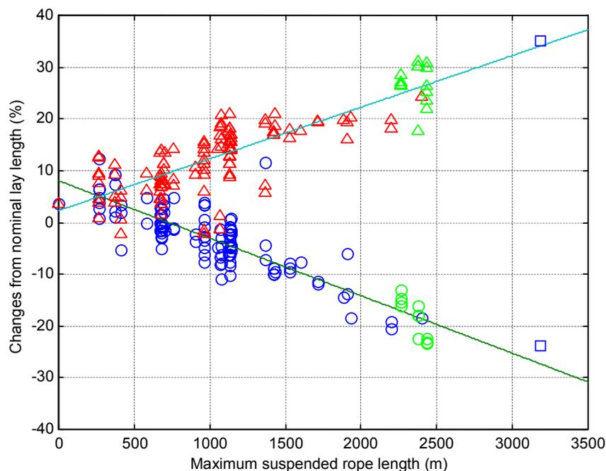
**Figure 3** - Installation lay lengths for 144 Lang's lay triangular strand ropes of varying rope diameter, construction and shaft depth. o = conveyance end,  $\Delta$  = sheave end,  $\square$  = independently calculated predictions for a future deep shaft at 3185 m.
