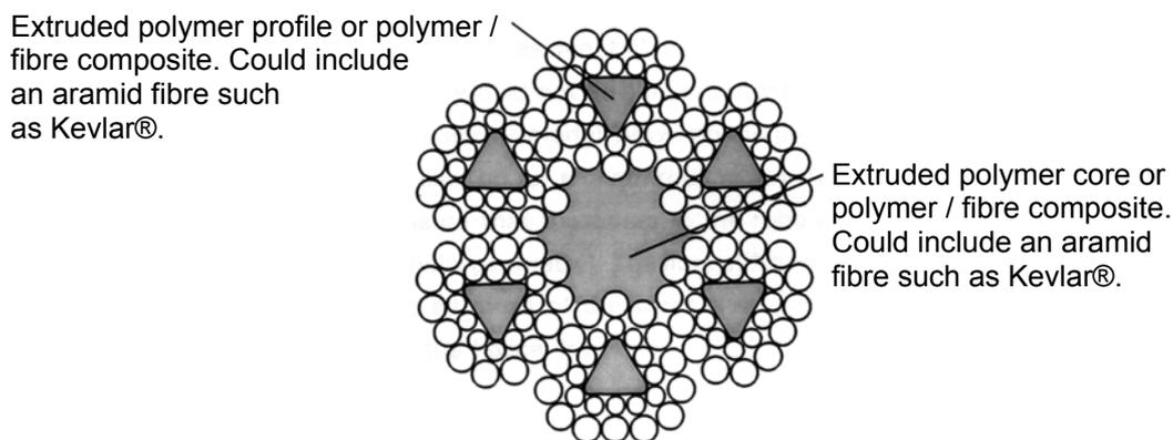
**Figure 10** - Option for reducing the weight of triangular strand ropes while maintaining the breaking strength and diameter. Adapted from Rebel<sup>1</sup> and McKenzie<sup>19</sup>.
