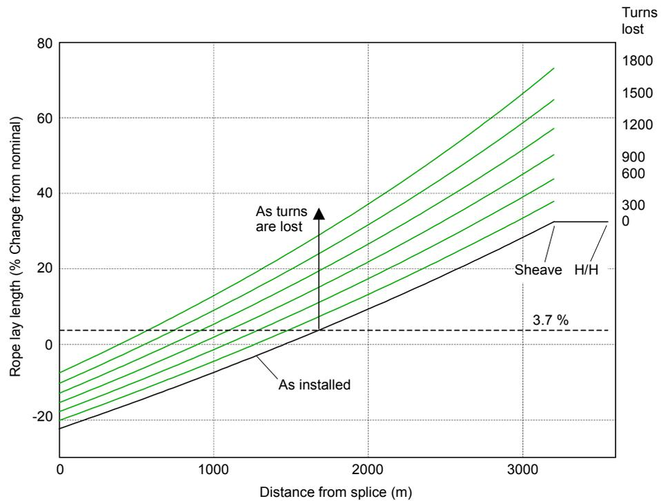
**Figure 9** - Example of the effect of lost rotation (in steps of 300 turns) on the distribution of in-service lay length changes for a 3200 m deep shaft. Note that the sheave end lay length increases more rapidly than at the splice end and becomes the area of concern as the service period progresses.
