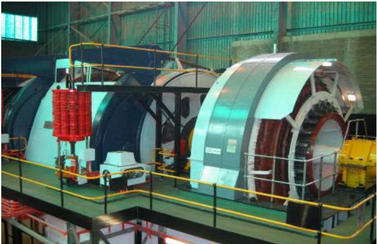
**Figure 1:** Driefontein No. 2 Shaft BMR Rock Winder. The winder has two separate 8,250 kW electrically coupled drum motors and each drum has two winding ropes.
