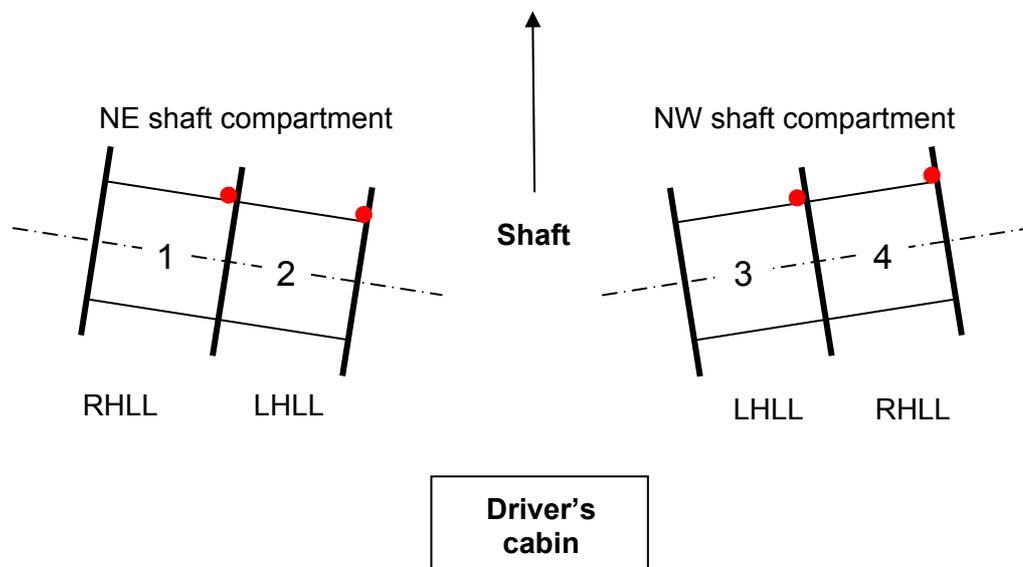
**NB:** both drums are overlay, red dots indicate positions of the hawse holes
