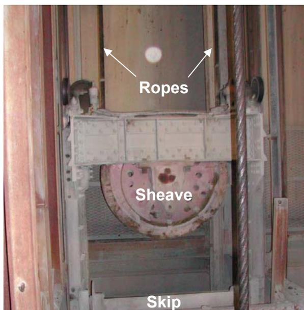
**Figure 3:** BMR rock winder rope load compensating sheave mounted on top of the skip.
