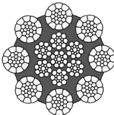
**Figure 6:** Typical round strand rope cross-section with compacted outer strands.
